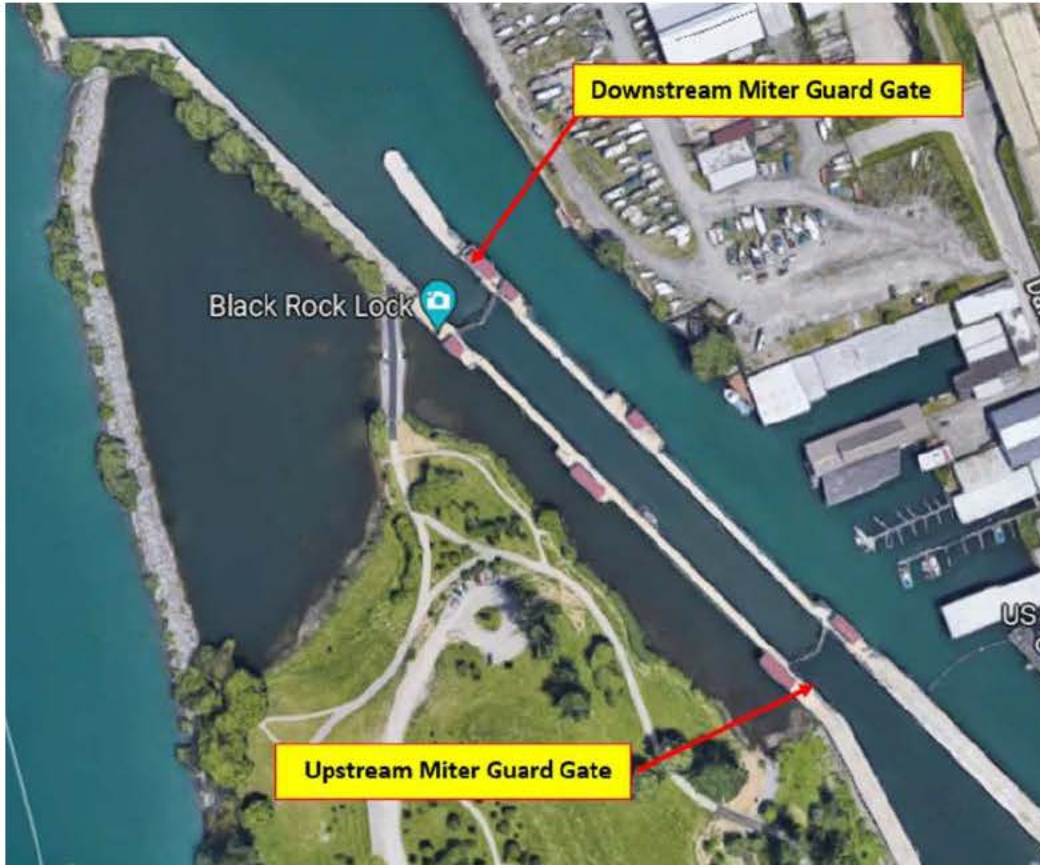
Figure 1. Black Rock Lock with Location of Miter Guard Gates Annotated
